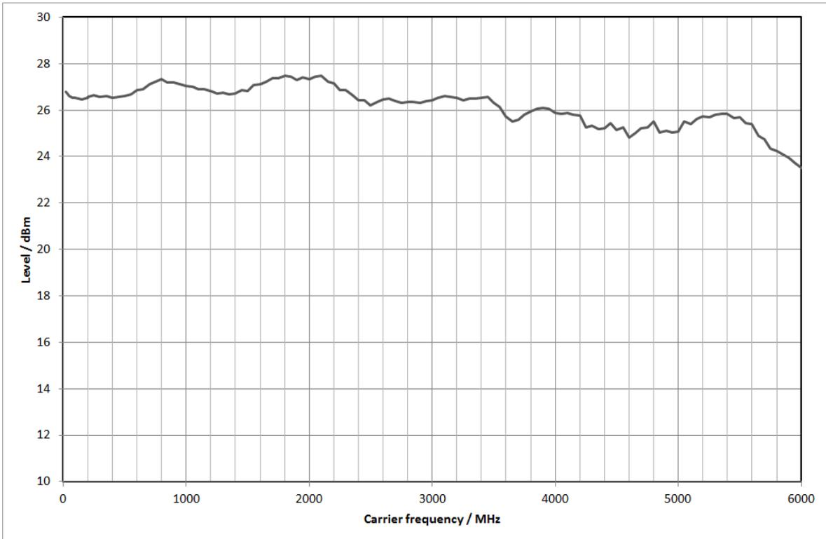
Measured maximum available output level versus frequency with R&S<sup>®</sup>SMW-B1006, R&S<sup>®</sup>SMW-B2006 frequency options
