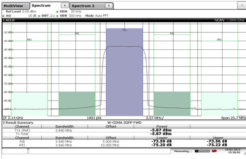
Measured ACPR for 3GPP test model 1, 64 DPCH
