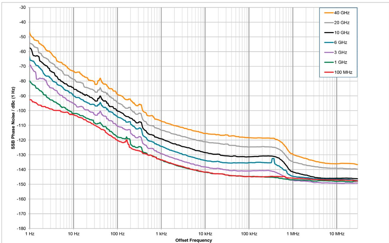
Measured SSB phase noise performance with R&S<sup>®</sup>SMW-B711/-B721 options, I/Q mode
