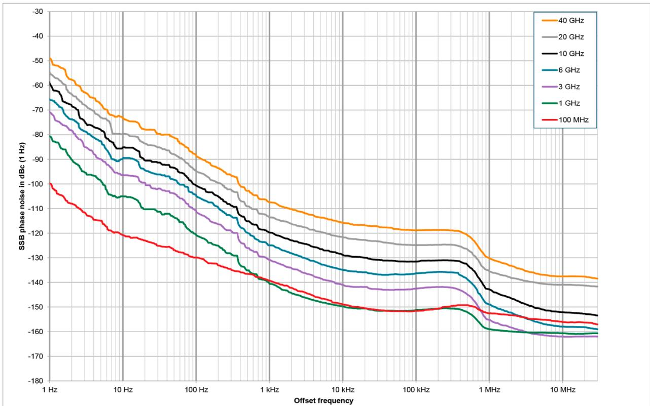
Measured SSB phase noise performance with R&S<sup>®</sup>SMW-B711/-B721 options, CW mode
