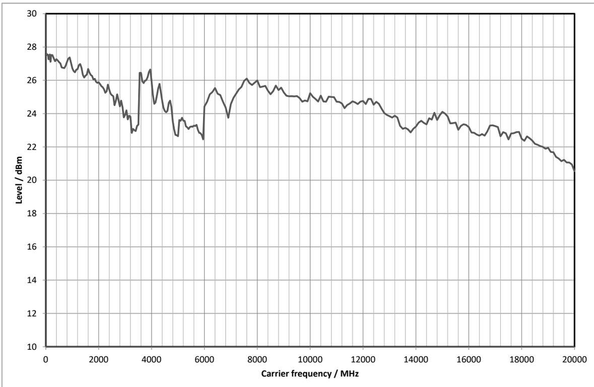
Measured maximum available output level versus frequency with R&S<sup>®</sup>SMW-B1020, R&S<sup>®</sup>SMW-B2020 frequency options
