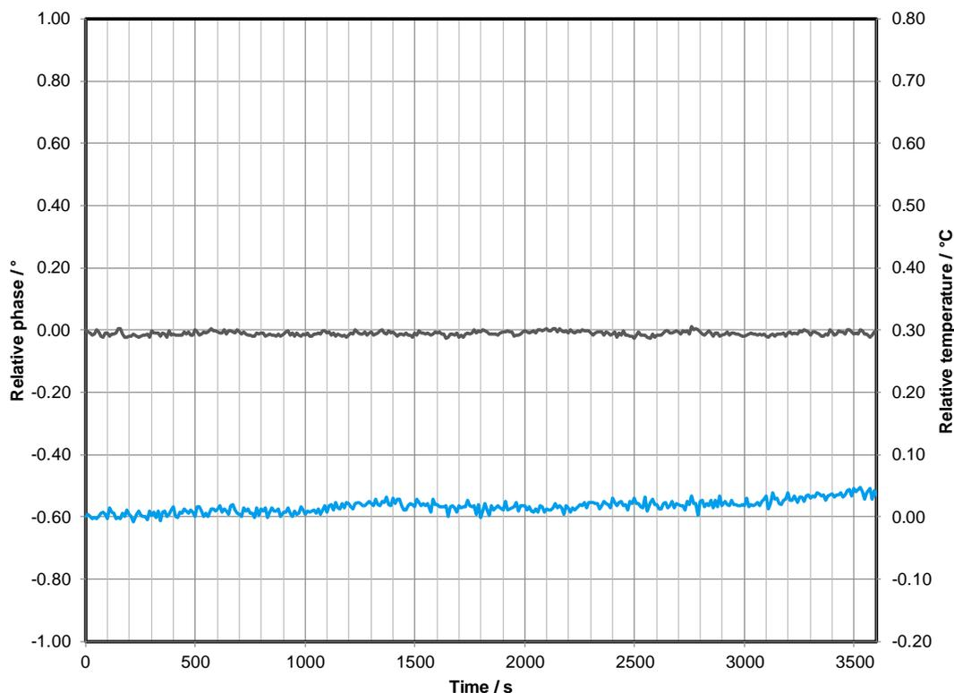
Measured relative phase between two LO coupled R&S<sup>®</sup>SMW200A RF paths vs. time, carrier frequency = 2 GHz, level = -10 dBm (the lower curve/right vertical axis indicates the temperature variation)
